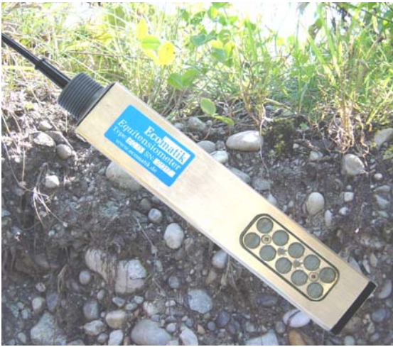
Type EQ15/Adapter: Equipped with screw adapter to connect with an extension tube, enabling deep soil installation
