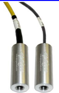
Original thermocouple output sensor with 6.5-14 μm window
